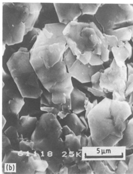
Figure 6 External views of the Na 2 -form of FZP. (a) 60°C, (b) 600°C, (c) 1000°C.
